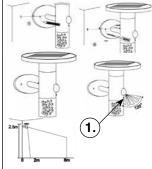
3. 3 different operating modes can be selected using the button below the PIR sensor (Fig. 1). The solar module should be covered. Proceed as follows:
