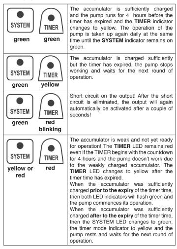
**Note:** When no operating mode is activated, then the output "PUMP" is switched off and the entire energy of the solar module flows into the accumulator.
